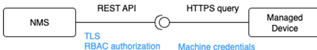
Figure 5.2.1-1: Secure channel example with TLS
