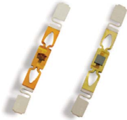
Figure 24: Smart RFID System on Alu strap
