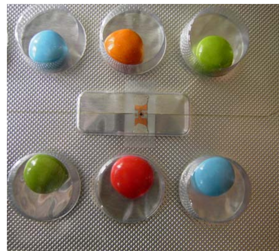
Figure 25: Polymer Strap on aluminium substrate with slot antenna
