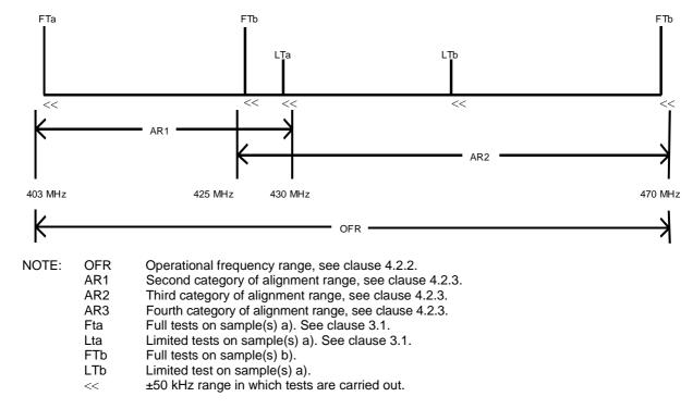
Figure D.3: Tests on family member equipment having alignment ranges that are subsets of the total operating frequency range - Example 1
