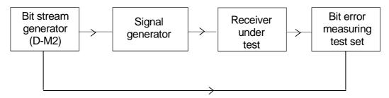
Figure 2: Measurement arrangement
