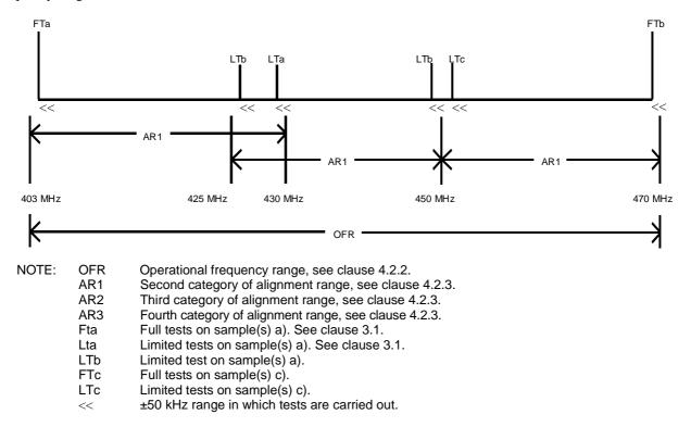
Figure D.4: Tests on family member equipment having alignment ranges that are subsets of the total operating frequency range - Example 2
