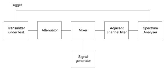
Figure 1: An example of a transient power measuring device measurement arrangement
