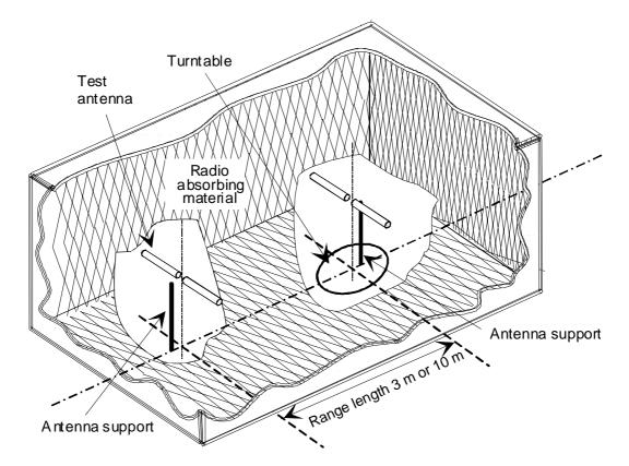
Figure A.1: A typical Anechoic Chamber
