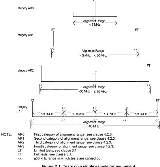
Figure D.1: Tests on a single sample for equipment that has a SR equal to its alignment range
