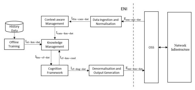
Figure 5-19: Mapping to ENI reference architecture (option two)
