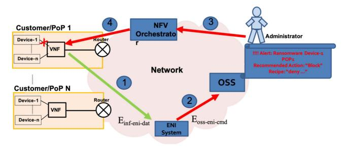
Figure 5-46: Use Case to limit profit in cyber-attacks using NFV and ENI system
