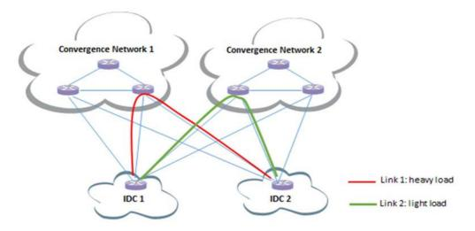
Figure 5-1: Policy-driven, automatic IDC traffic steering
