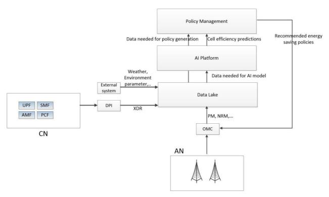
Figure 5-6: Energy saving for radio network
