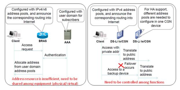
Figure 5-7: Current Problems in Operator IP Managed Networks
