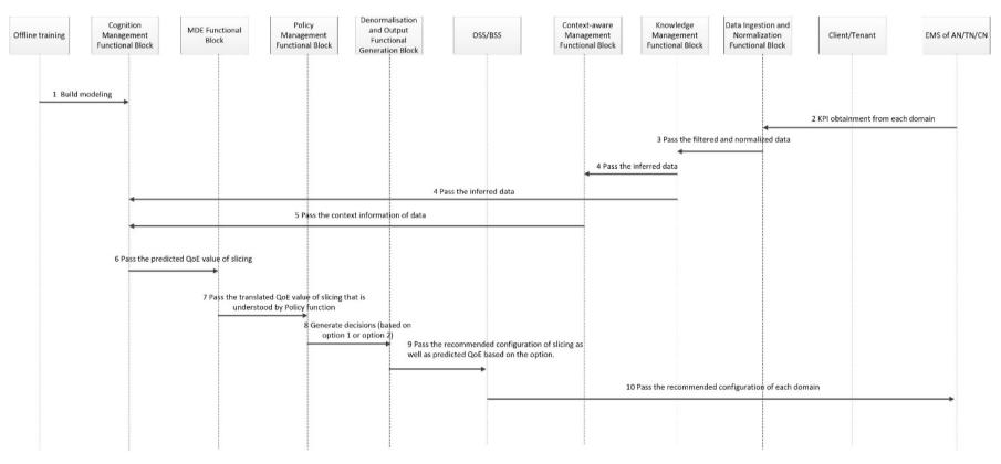
Figure 5-35: Flow of information for "service experience optimization of E2E slicing involving both BSS and OSS"
