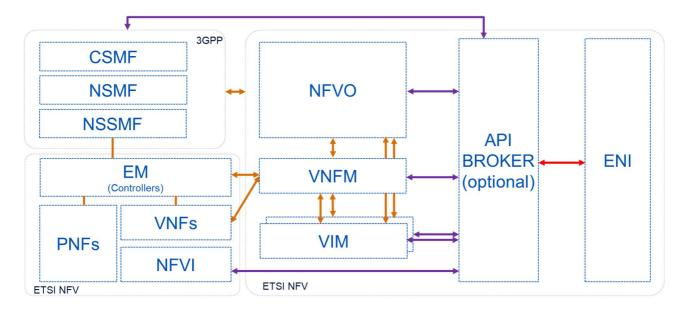
Figure 5-12: An architectural design including ETSI NFV MANO, 3GPP management functions, and ENI engine
