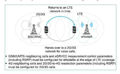
Figure 5-27: Interoperability between VoLTE and 2G and 3G
