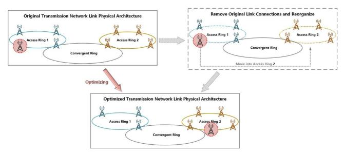
Figure 5-5: Original and Optimized Transmission Network Link Physical Architecture
