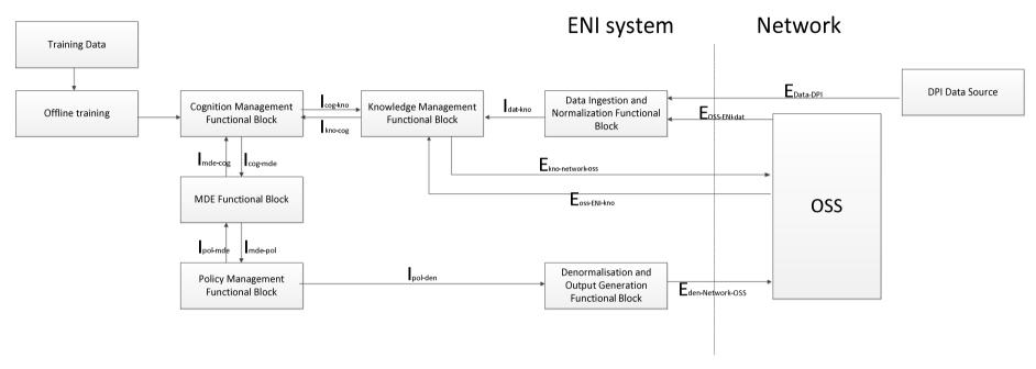
Figure 5-15: Mapping to ENI reference architecture for Application Characteristic based Network Operation
