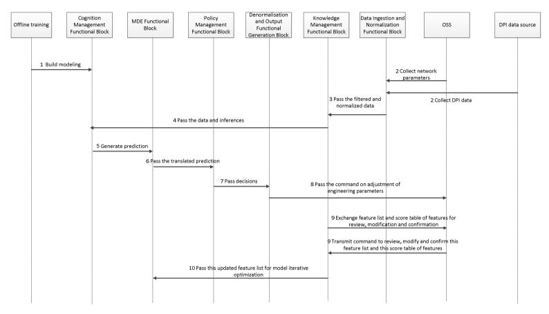
Figure 5-16: Flow of information for Application Characteristic based Network Operation
