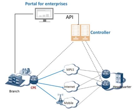
Figure 5-31: Intelligent carrier managed SD-WAN service
