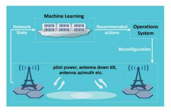
Figure 5-8: Coverage and Capacity Optimization
