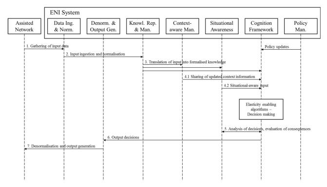
Figure 5-13: Example Flow of information among the ENI System's functional blocks and the Assisted System
