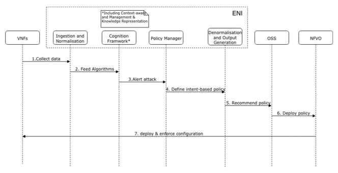
Figure 5-47: Flow of information among the ENI System's functional blocks and the Assisted System
