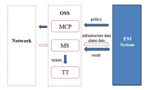
Figure 5-44: Scenario of AI and ENI system enabled network fault root-cause analysis and intelligent recovery
