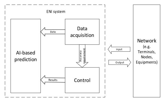
Figure 5-24: Intelligent time synchronization of network
