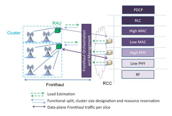
Figure 5-11: Concept of the proposed Fronthaul use case
