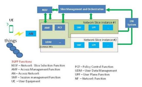
Figure 5-30: Example of a network slicing management and orchestration scenario
