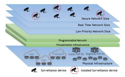
Figure 5-45: Device isolation within a Network Slice
