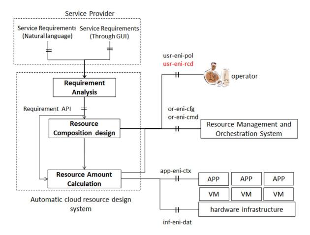
Figure 5-23: Automatic Cloud Resource Design System
