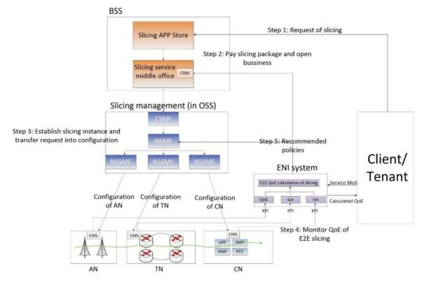
Figure 5-33: Possible deployment scenario of Service experience optimization of E2E slicing involving both BSS and OSS
