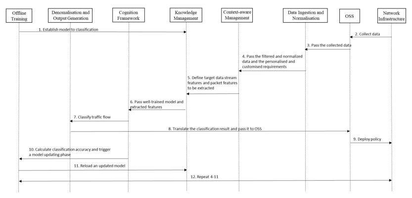
Figure 5-20: Scenario of AI enabled network traffic classification (option one)
