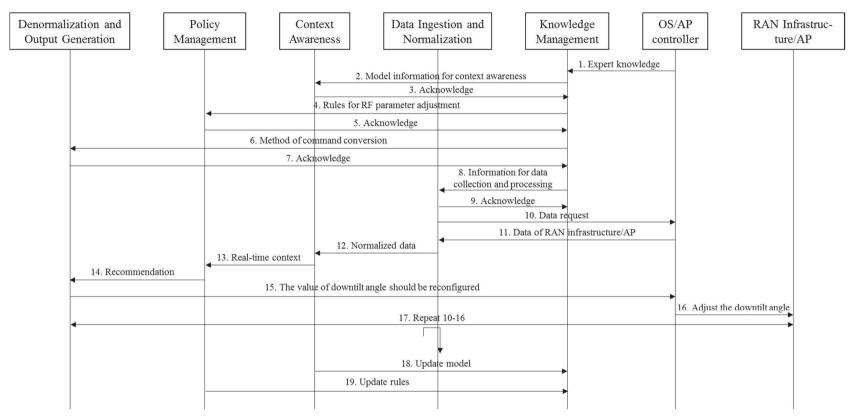
Figure 5-10: Procedure for coverage and capacity optimization
