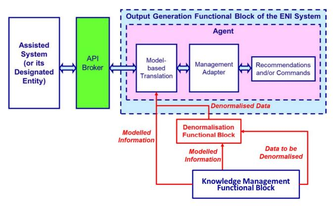
Figure 6-37: Output Generation Operation
