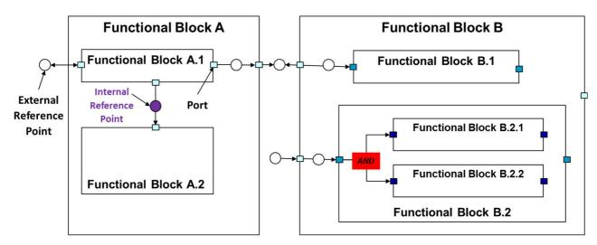
**Figure 6-1: Functional Block Notation**
