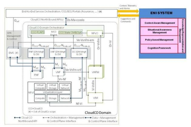
Figure A-1: Interaction between the BBF CloudCO and ENI
