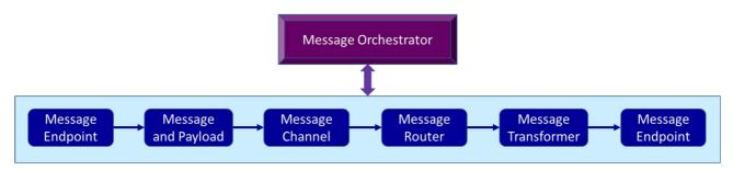
Figure 6-39: Functional Block Diagram of an ENI Messaging System
