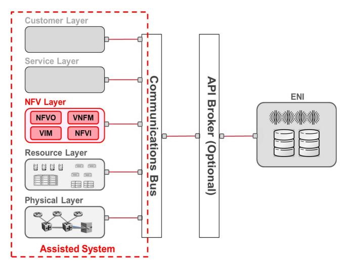
Figure 9-2: Interaction between the NFV MANO and ENI
