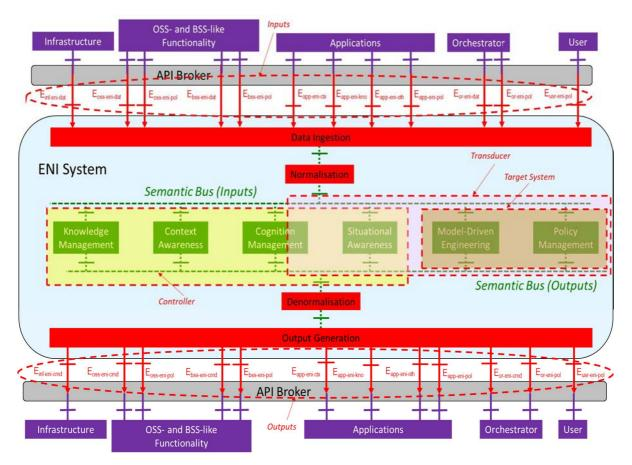
Figure 6-11: Functional Architecture with Exemplary Control Loops
