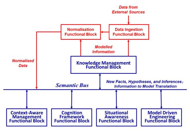
Figure 6-14: Data Normalization Operation
