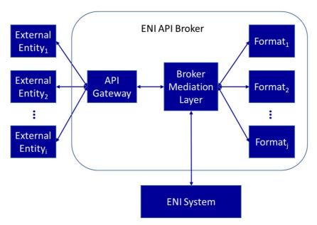
Figure 6-38: Function of the ENI API Broker
