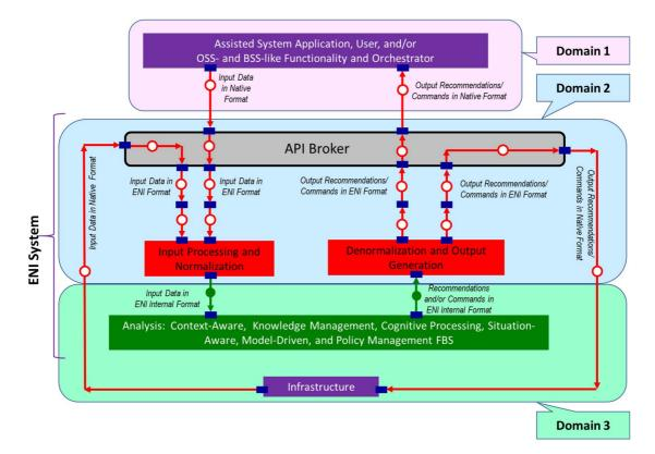
Figure 6-10b: Functional Architecture with Exemplary Internal Domains
