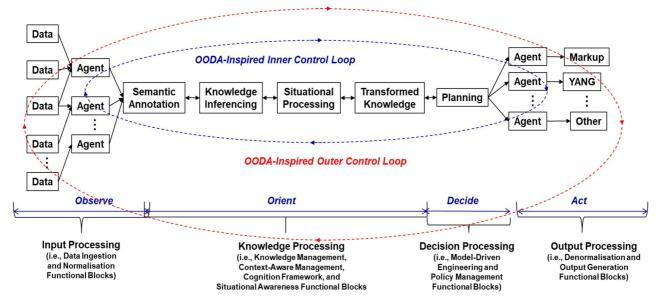
Figure 6-18: Simplified Knowledge Processing Flow
