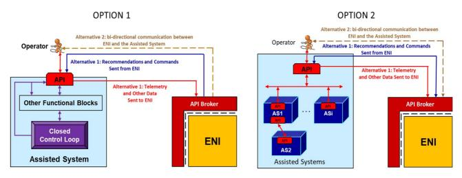
Figure 4-4: Class 3: Assisted System with AI in the Control Loop
