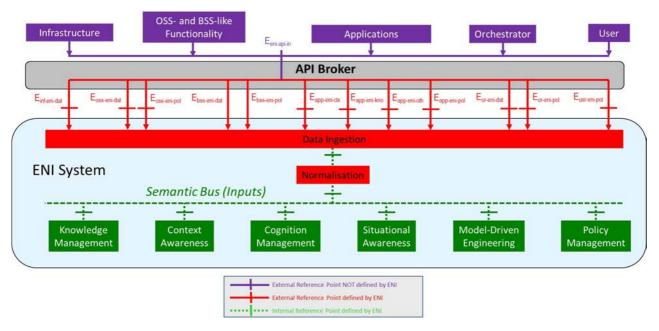
Figure 6-7: Functional Architecture with its Input Reference Points
