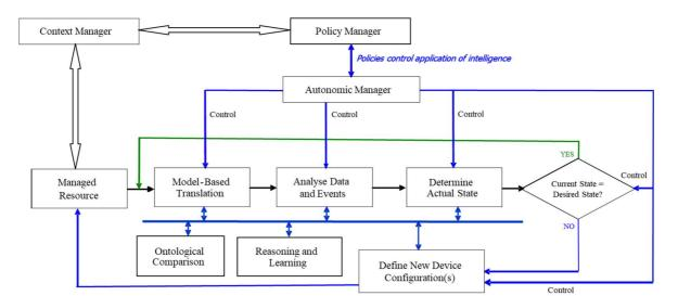
Figure 6-35: Simplified Functional Block Diagram of the FOCALE Architecture
