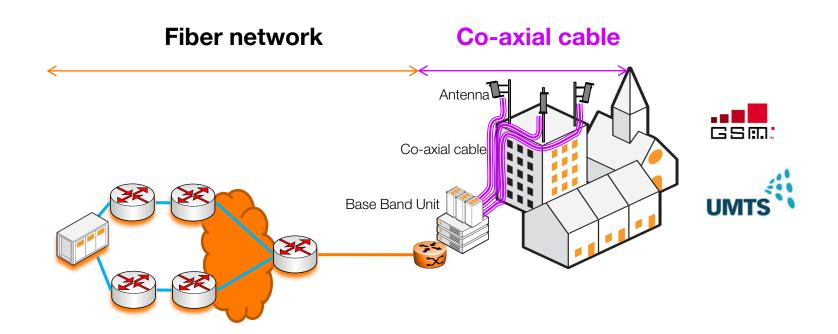
Legacy backhaul is based on PtP Ethernet (Switch or Router connected at a dark fiber)
