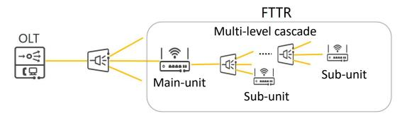
Multi-level non-uniform: The end-to-end maximum optical link loss needs to be recalculated
