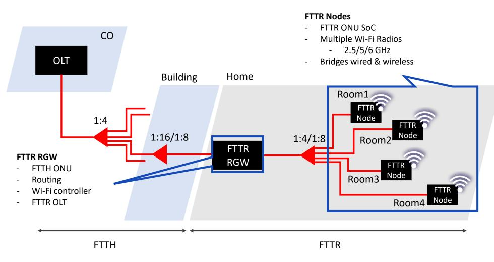
FTTR could complement current deployment options by providing a robust, low latency and high throughput Wi-Fi backhauling option for:
