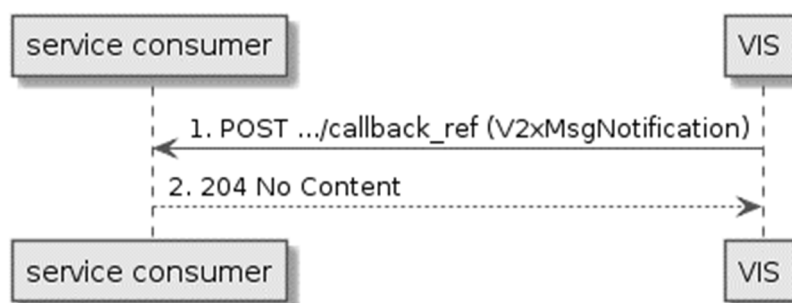
Figure 5.5.10.3-1: Flow of V2X message notification
