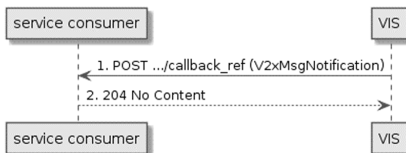
Figure 5.5.10.3-1: Flow of V2X message notification
