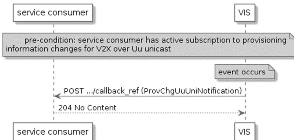
Figure 5.5.7-1: Flow of receiving V2X information event notifications about the provisioning information changes for V2X communication over Uu unicast
