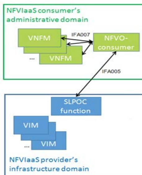
**Figure 5.2.5-1: Illustration of NFVIaaS architecture option 2.b**
