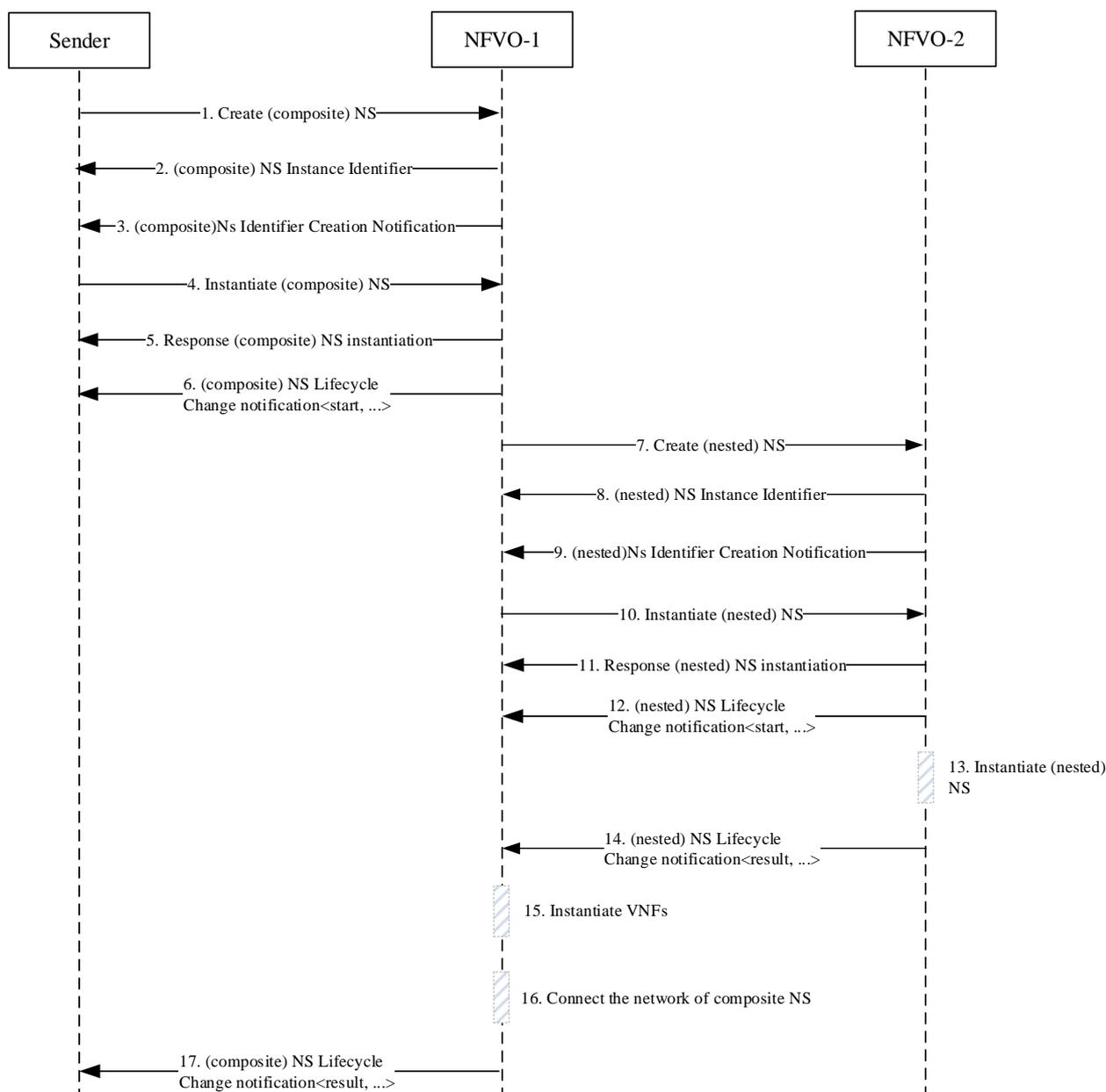
**Figure A.1.2a-1: Top-down Composite NS instantiation**
