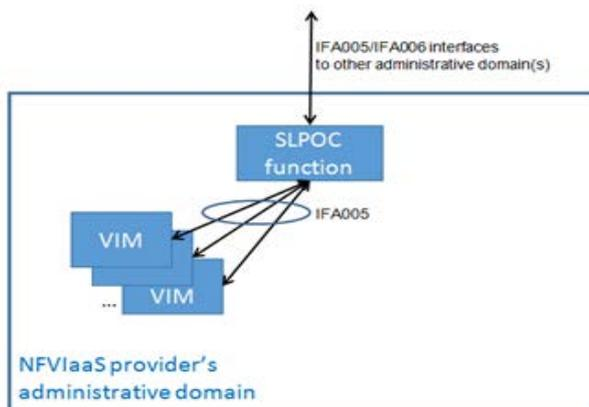
**Figure 5.2.4-2: Illustration of SLPOC interfaces**
