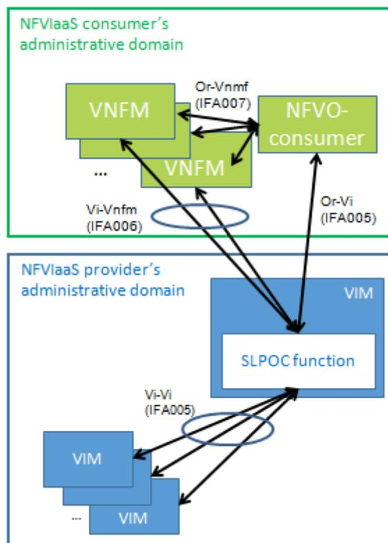
**Figure 5.2.7-1: Illustration of SLPOC function integrated into VIM**
