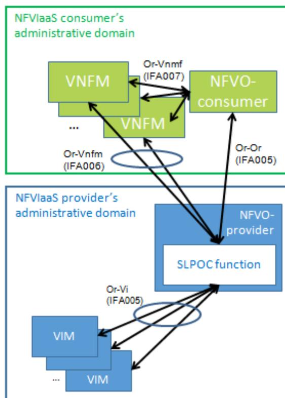
**Figure 5.2.7-2: Illustration of SLPOC function integrated into NFVO**
