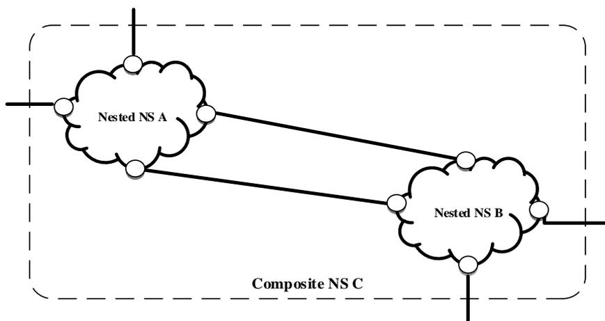
**Figure 6.1-1: Composite NS and nested NSs example**
