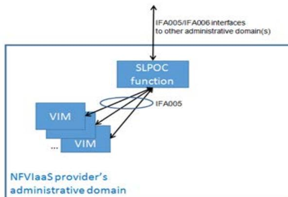
**Figure 5.2.5-2: Illustration of SLPOC interfaces**
