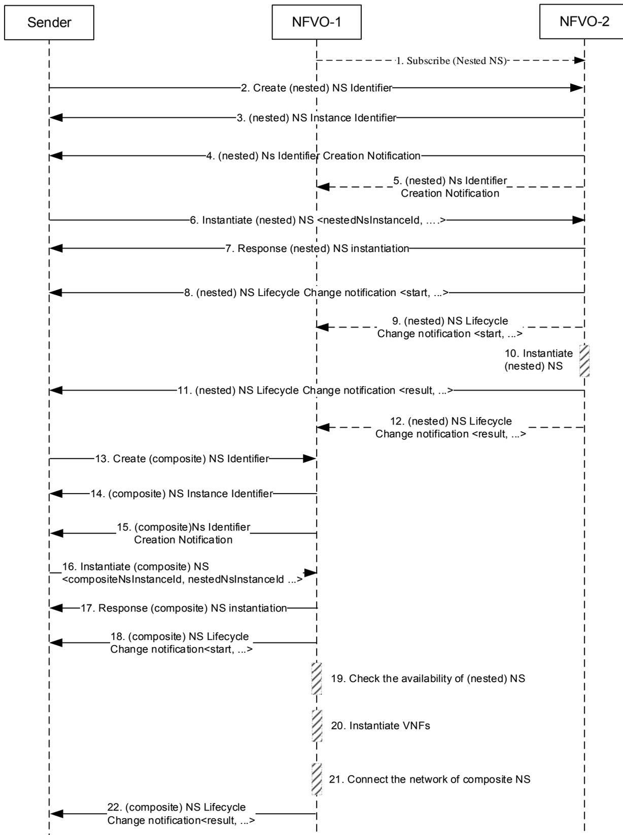
Figure A.1.5-1: Bottom-up Composite NS instantiation
