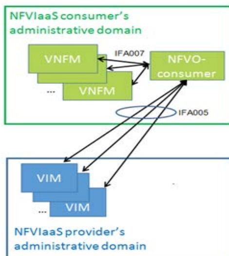
**Figure 5.2.3-1: Illustration of NFVlaaS architecture option 1.b**
