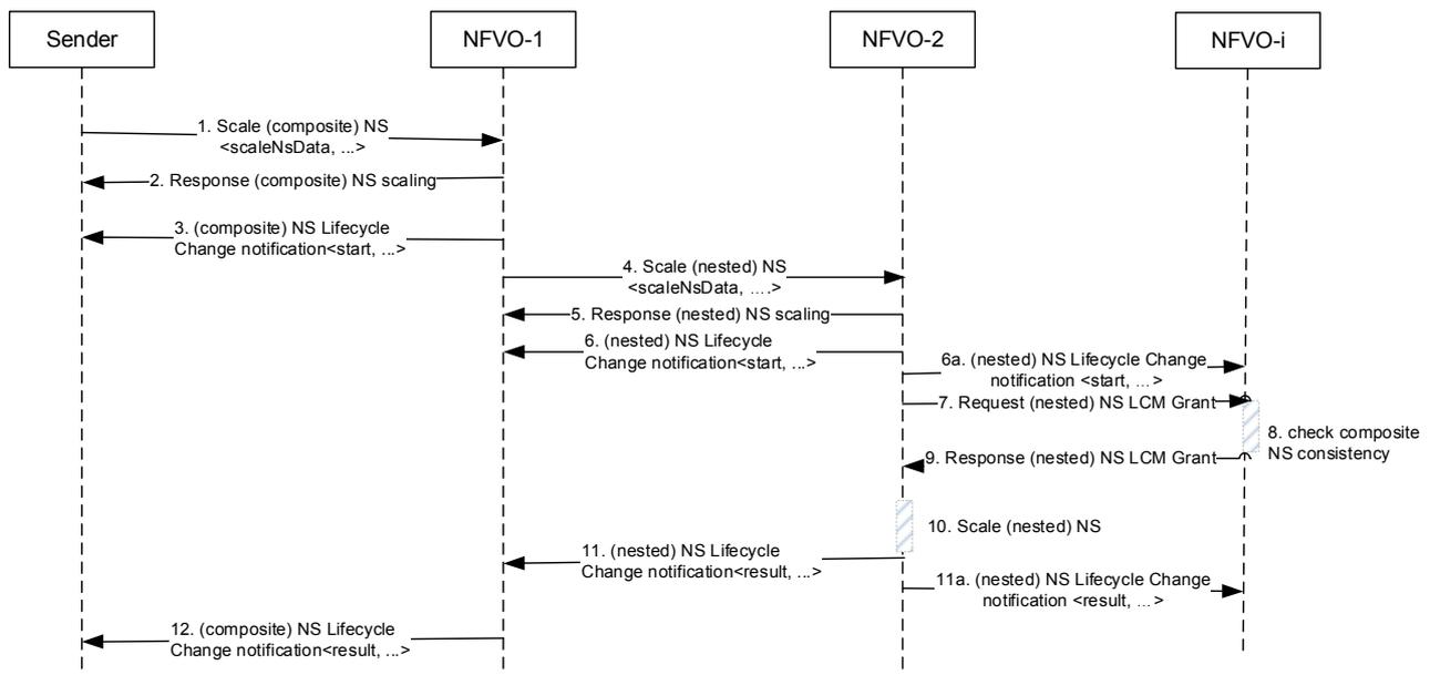
Figure A.1.3b-1: Composite NS scaling in sharing scenario
