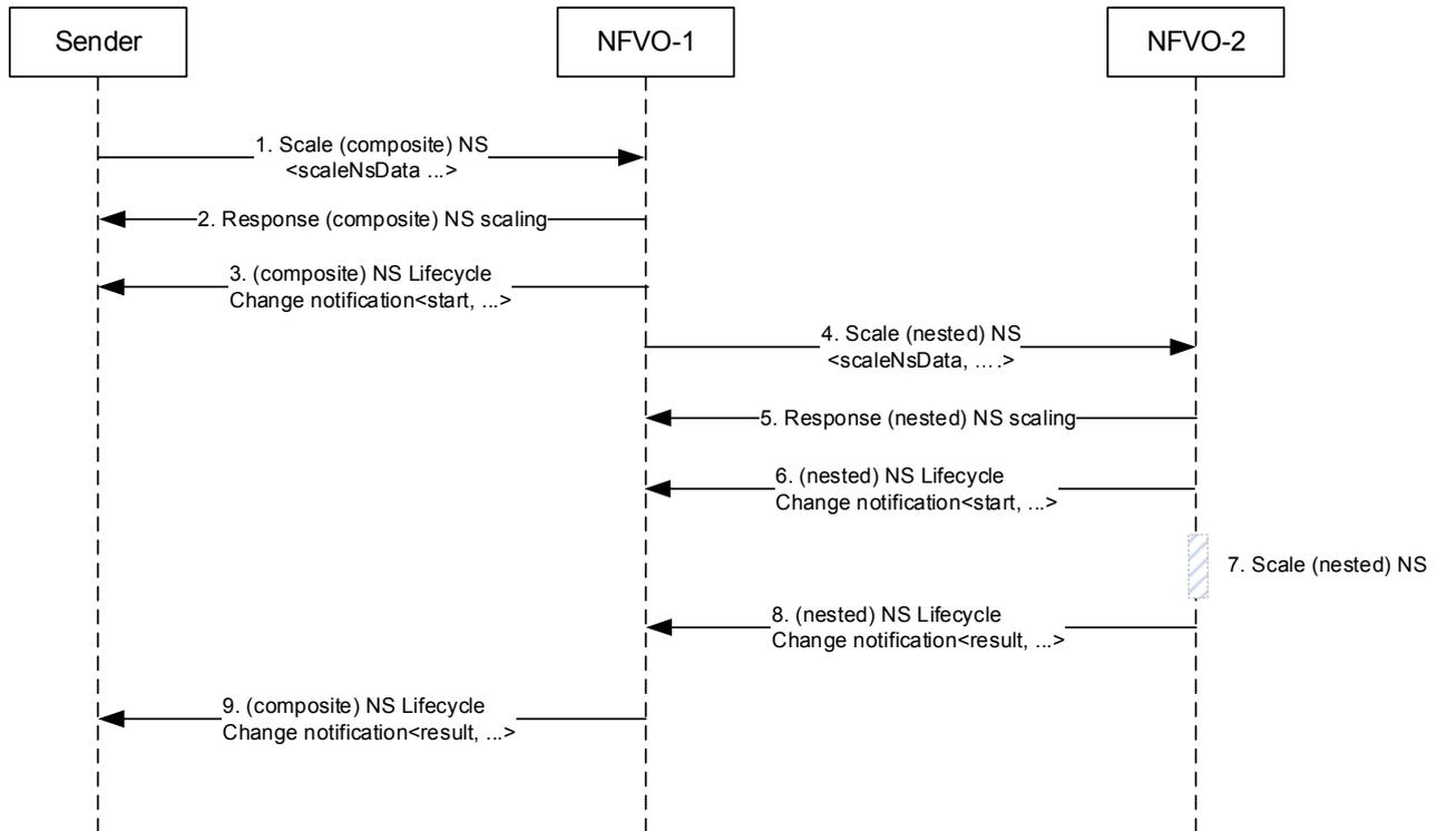
**Figure A.1.3a-1: Composite NS scaling**
