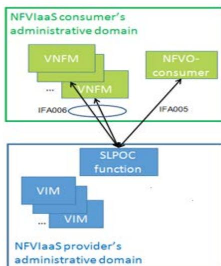
Figure 5.2.4-1: Illustration of NFVIaaS architecture option 2.a
