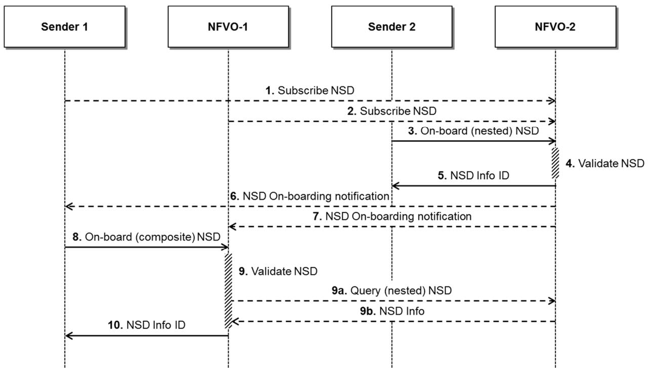
**Figure A.1.1-1: Composite NSD on-boarding flow**
