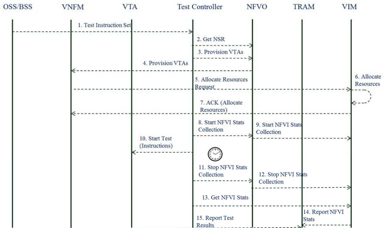
**Figure 4: Message Sequence Flow for Active Monitoring**
