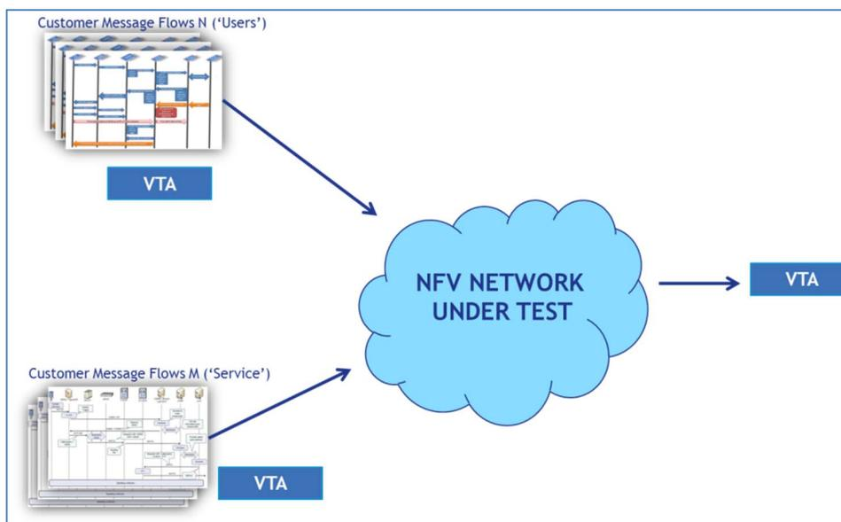
**Figure 14: Example Topology for capacity validation**
