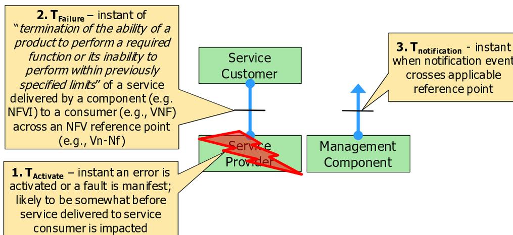
**Figure 8: Canonical Failure Notification Model**
