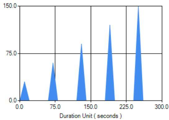
**Figure B.3: Burst Load Pattern**
