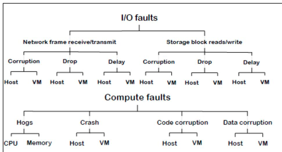
Figure 23: Faultload for the dependability evaluation of NFVI
