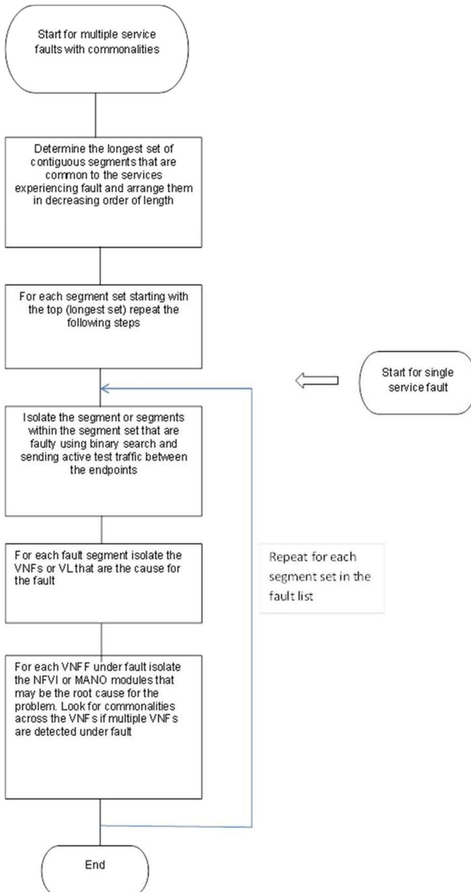
Figure A.2: Example Fault Isolation Workflow
