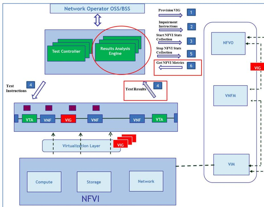
Figure 20: Fault injection framework in conjunction with active monitoring
