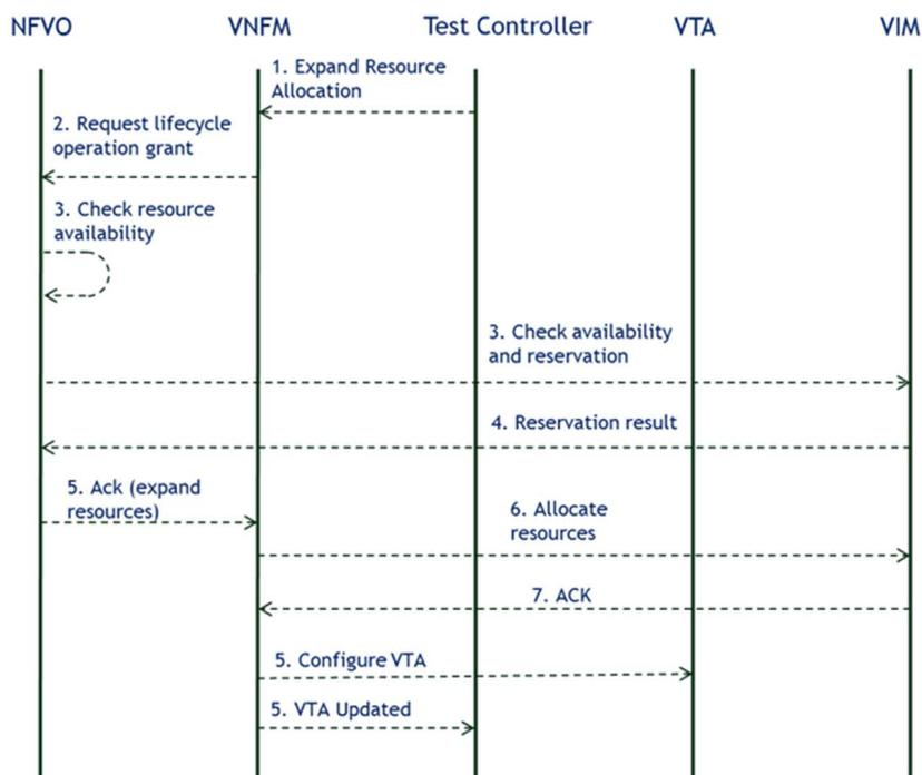
**Figure 5: Expansion of NFVI resource allocations for VTA**
