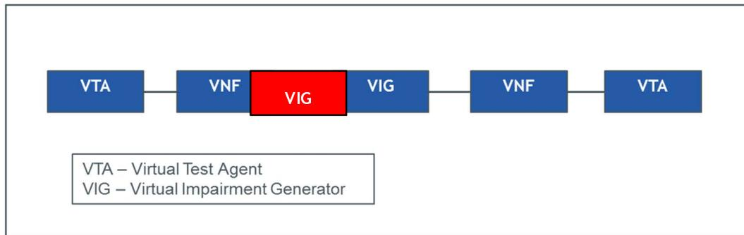
**Figure 24: Fault injection using virtual impairment generator**
