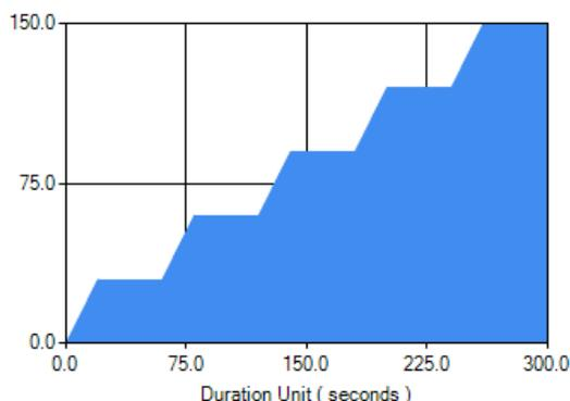
Figure B.1: Staircase Load Pattern
