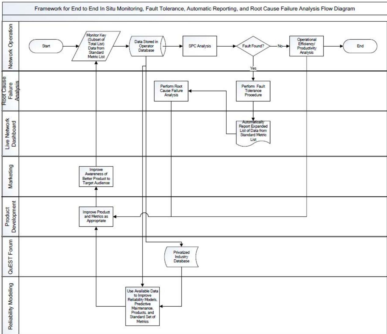
Figure 13: Process Workflow
