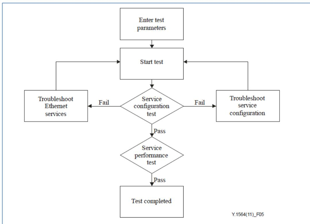
**Figure 10: High level test methodology for service activation
