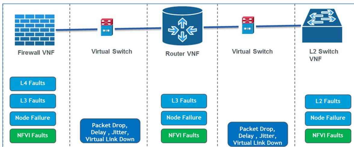
Figure 22: Challenge levels based on VNF type
