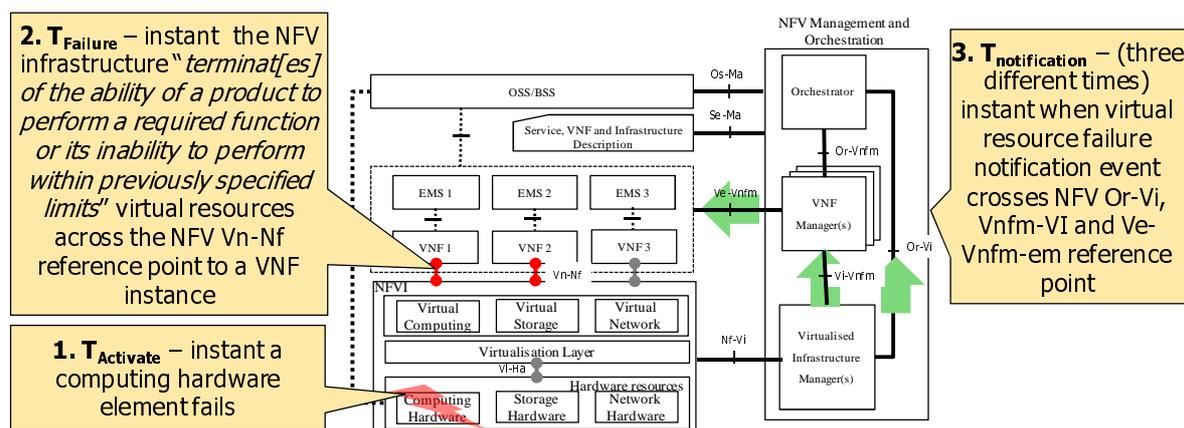
Figure 9: Use Case of Canonical Failure Notification Model
