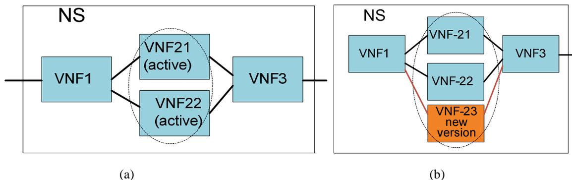
NOTE: (a) with load sharing (b) and adding a VNF instance of the new software version into the NS.
