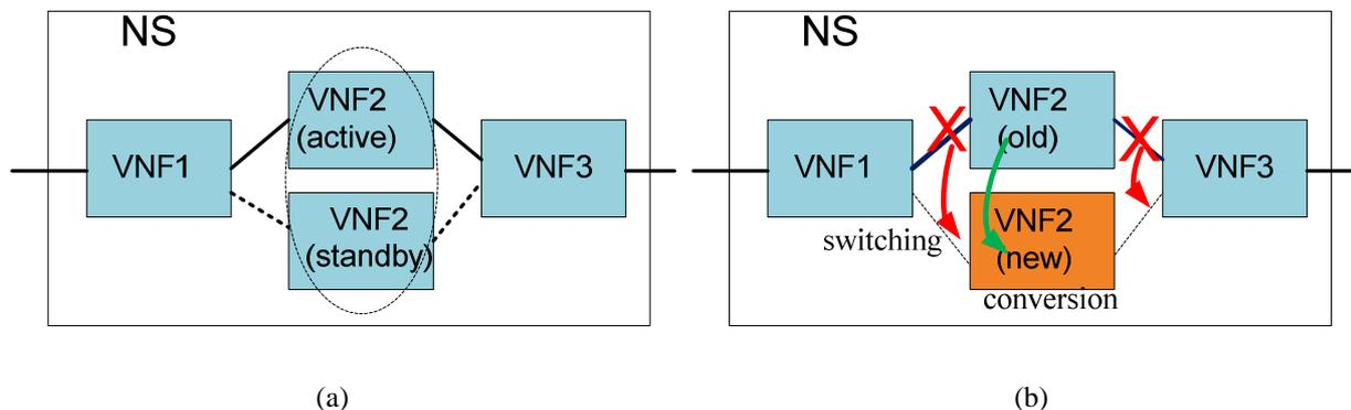
NOTE: (a) in an active-standby configuration (b) and their rolling upgrade by upgrading one VNF instance at a time.
