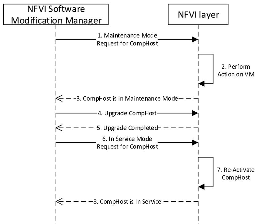
**Figure C.2: Example Handling of NFVI Resource Software Modification**
