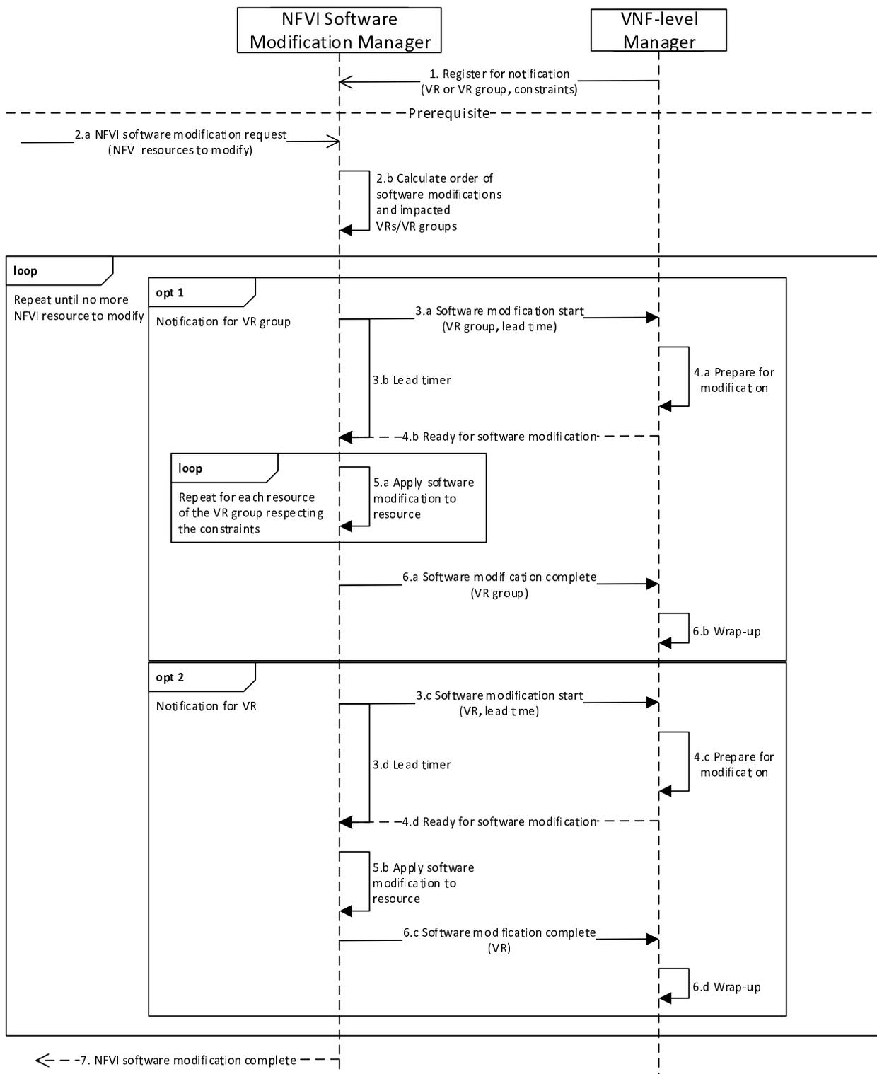
Figure C.1: Exemplary coordination flow for NFVI software modification
