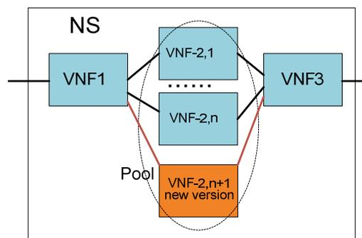
**Figure A.1: Diagram of a stateless VNF software upgrade**
