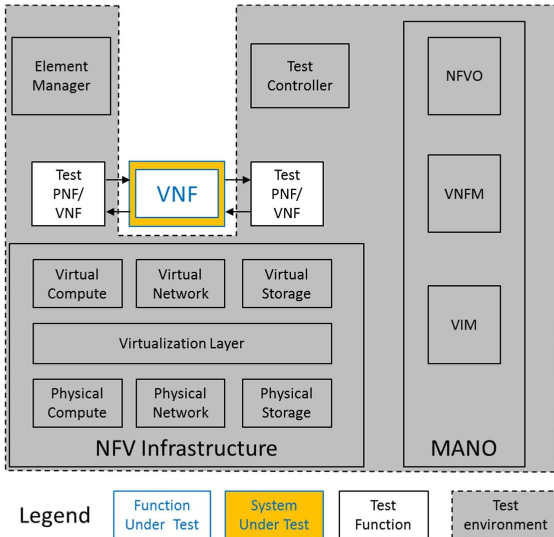
**Figure 4.3: Functional architecture for VNF Under Test**
