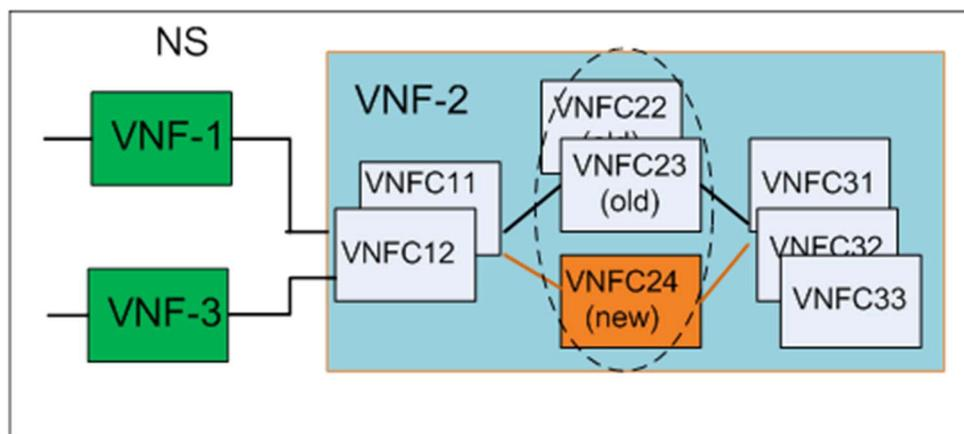
NOTE: Type 1 VNFC: VNFC11 and VNFC12 as redundancy pairs; Type 2 VNFC: VNFC22 and VNFC23 as a load sharing pool; Type3 VNFC: VNFC31, VNFC 32 and VNFC33 as another load sharing pool.
