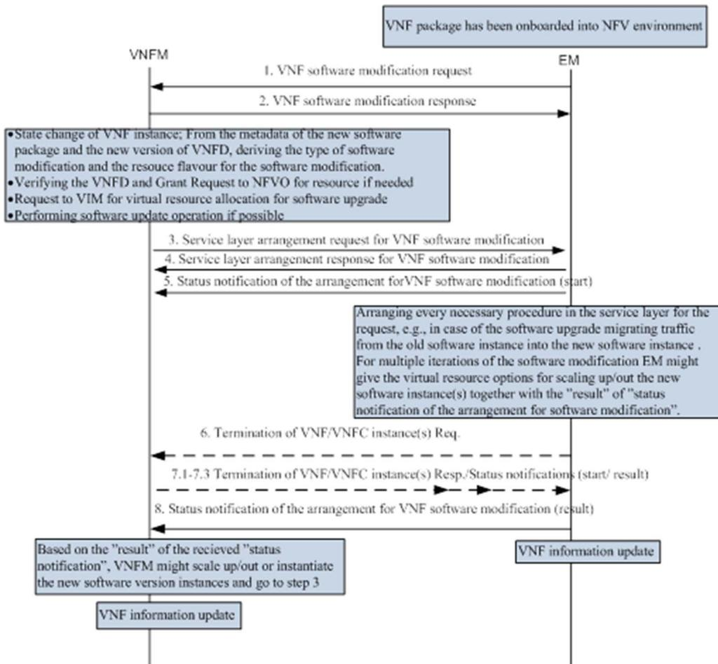
Figure B.2: Flow diagram for the operation of the VNF software modification initiated from EM
