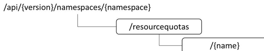
**Figure 11.3-6: Resource URI structure of ResourceQuotas object for the OS container configuration management service interface**
