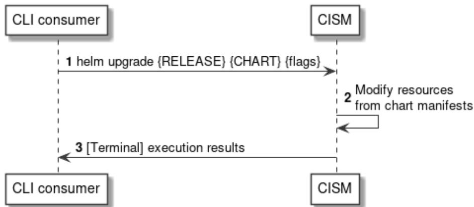
**Figure 7.3.2-1: Flow of containerized workload modification via upgrade**
