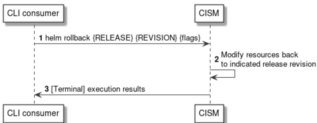
**Figure 7.3.3-1: Flow of containerized workload modification via rollback**
