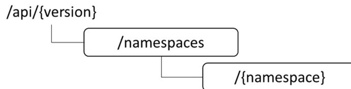
**Figure 11.3-5: Resource URI structure of Namespace resource object for the OS container configuration management service interface**
