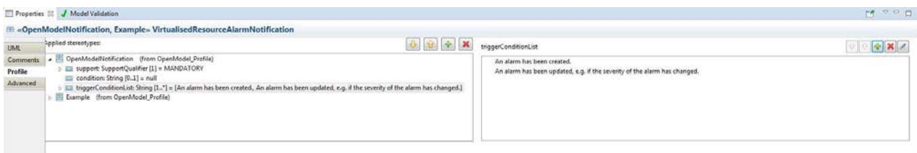
Figure 5.7.3-2: Notification trigger condition list
