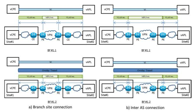
Figure 5.2.7.3-1: Mapping of service instance Model to infrastructure related to an E2E EvCPE service across WAN
