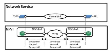
Figure 5.2.1-1: Connectivity overview for enabling Network Service
