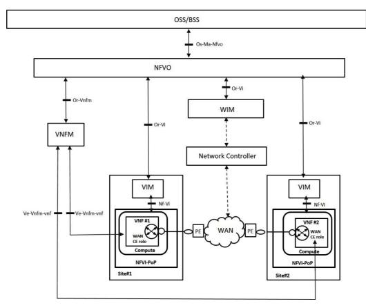
Figure 5.14.1-2: High level use case of WAN connectivity in compute-only NFVI-PoPs
