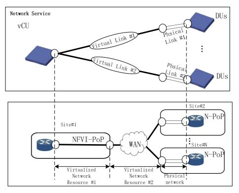
Figure 5.13.1-1: Connectivity overview for enabling Network Service
