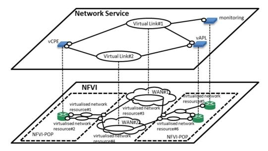
Figure 5.3.1-1: Connectivity overview for enabling End-to-End Network Service across two WANs
