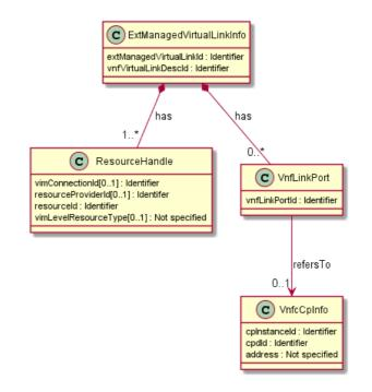
Figure 6.4.4.2.1-1: Extension to support multiple ResourceHandle to realize an ExtManagedVirtualLinkInfo
