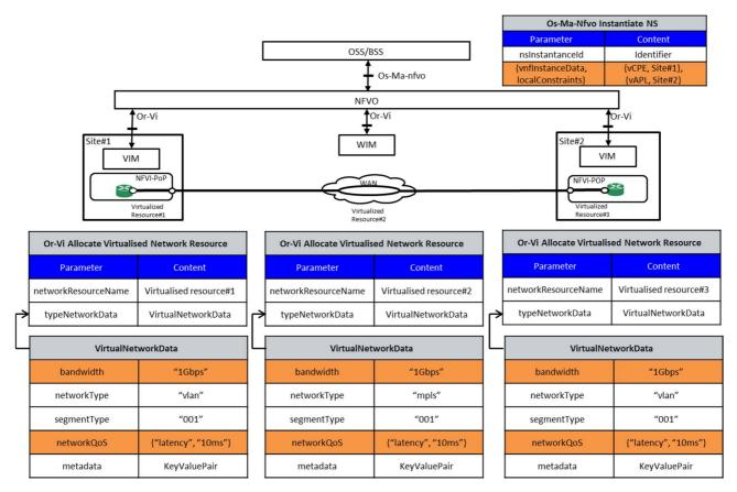
Figure 5.2.7.4-2: Mapping of service instance Model to infrastructure related to an E2E EvCPE service across WAN
