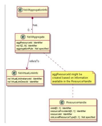
Figure 6.4.3.2.1-1: Option #1 for NS VL aggregation
