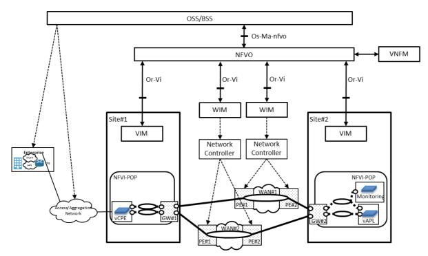
Figure 5.3.1-2: High-level use case for an E2E EvCPE service across two WANs
