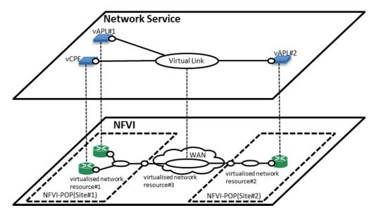
Figure 5.4.1-1: Connectivity overview for enabling NS expansion over WAN
