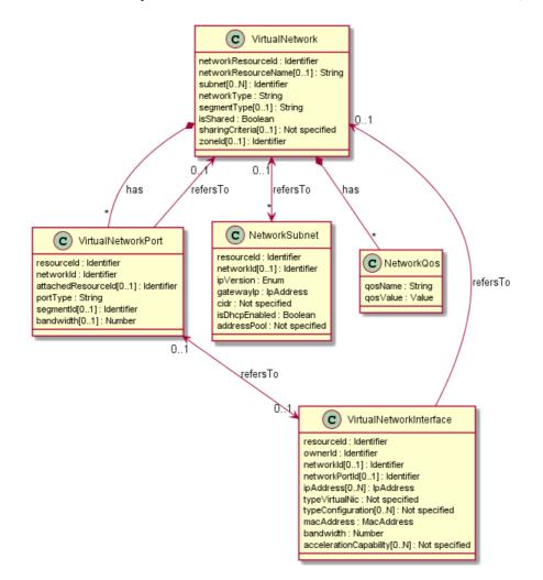
Figure 6.4.5.1-1: Current VirtualNetwork information model from ETSI GS NFV-IFA 005 [i.7]
