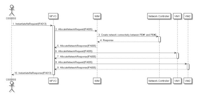
Figure 5.2.7.4-1: Instantiate a connectivity service
