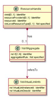
Figure 6.4.3.2.1-3: Option #3 for NS VL aggregation
