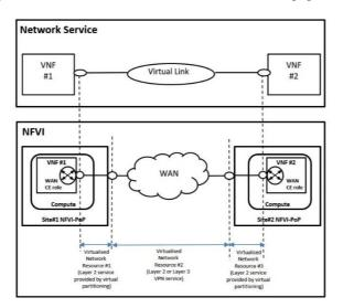
Figure 5.14.1-1: Connectivity overview of Network Service in compute-only NFVI-PoPs
