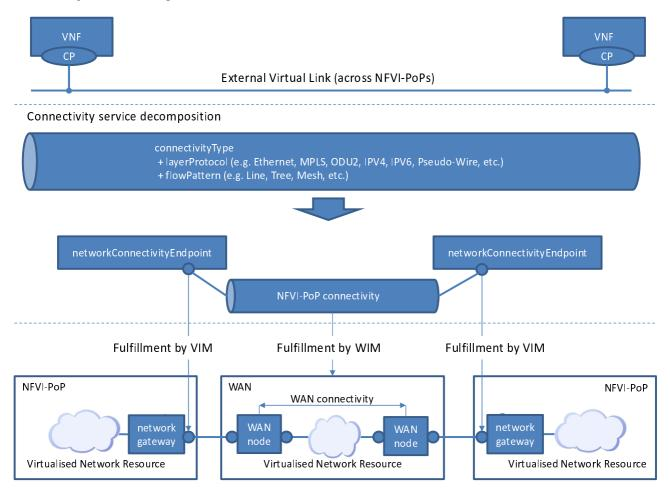
Figure 6.2.2-1: Mapping and decomposition of connectivity service
