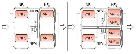
a) Input load below the scaling threshold b) Input load over the scaling threshold
