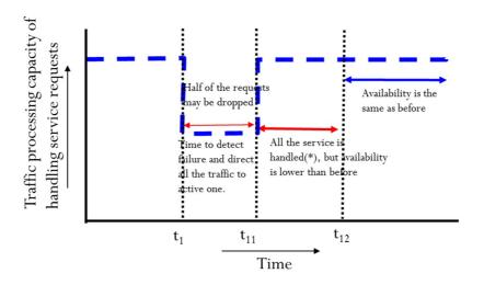
(b) An example of traffic processing capacity change for providing service in remediation/recovery after a failure occurs (Active-Active configuration).
