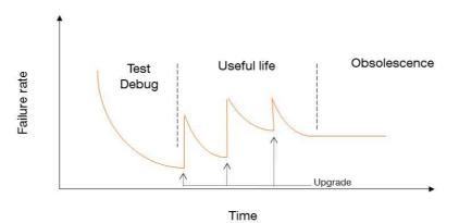
Figure 5: Software failure rate
