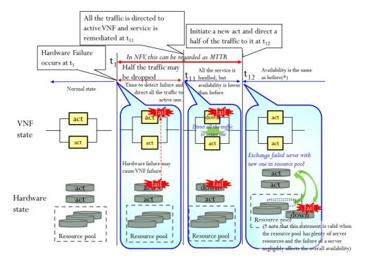
(a) Situation after a hardware failure occurs at a server on which one of the active VNFs resides.
