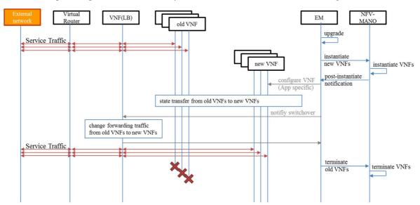
Figure 54 shows a possible procedure controlled by the EM, where traffic is distributed among VNF instances.
