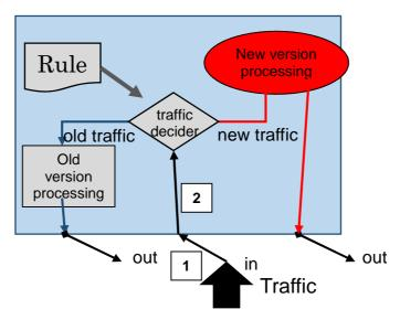
Figure 71: A diagram of traffic routing during software upgrade
