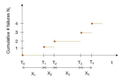
Figure 8: Failures process
