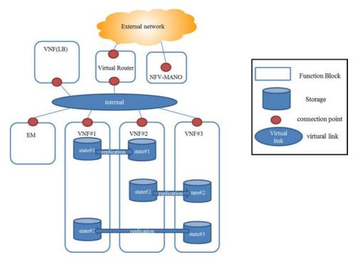
Figure 46: Load balancing model with internal storage
