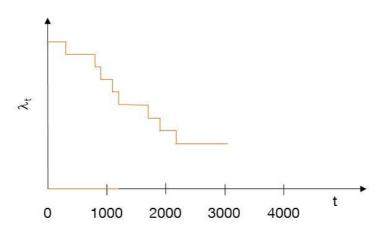
Figure E.1: Jelinski-Moranda failure intensity
