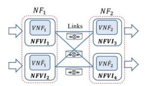
Figure 60: Active-Active redundancy for all elements of a sub network
