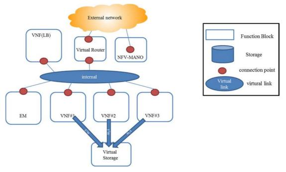
Figure 52: Load balancing model with virtual storage
