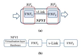
Figure 55: (a) A sub network SN1 using a single NFVI and (b) its reliability block diagram
