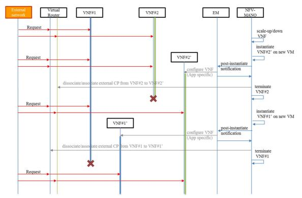
Figure 43: A scale up/down procedure of VNFs synchronizing state information in the Active-Active configuration
