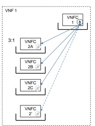
Figure 23: n:1 (3:1 shown) Active-Standby with externalised state push/pull (no state replication of underlying VNFCIs); remediation to state determined by controlling VM
