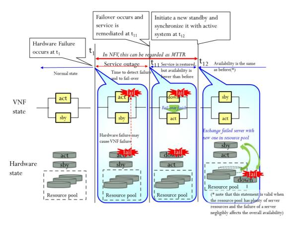
(a) Situation after a hardware failure occurs at a server on which the active VNF resides.
