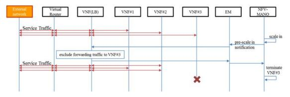
Figure 49: A possible scale-in procedure of a VNF in the load balancing model (stateless)
