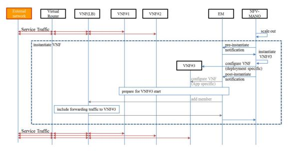
Figure 51: A possible scale-out procedure of a VNF in the load balancing model (stateful)
