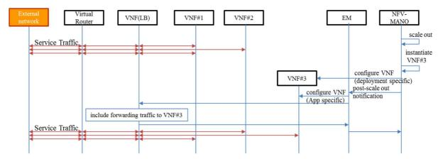
Figure 48: A possible scale-out procedure of a VNF in the load balancing model (stateless)
