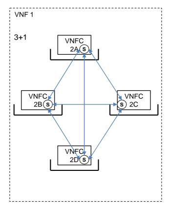
Figure 28: N+M example, 3+1, working with direct partial VM mesh state replication; stateful remediation
