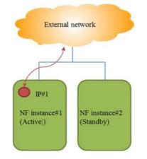
Figure 29: An Active-Standby configuration of NFs
