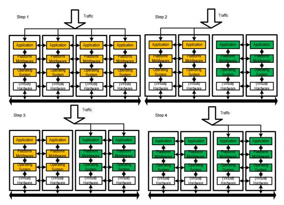
Figure 69: Main steps of software upgrade procedures (without redundancy) in a traditional network function
