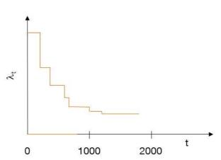
Figure E.2: Failure intensity of the geometric model
