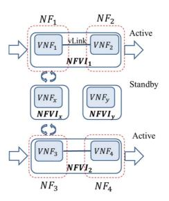
Figure 62: N:M Active-Standby configuration (N=2, M=1)
