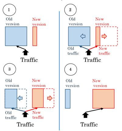
Figure 70: High level view of VNF software upgrade procedure
