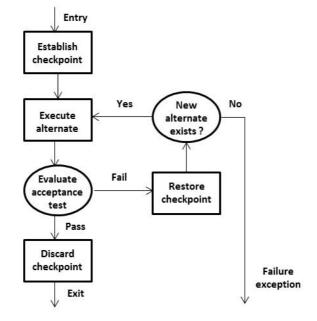
Figure 7: Operation of the recovery blocks
