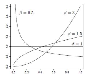
Figure E.3: Failure intensity of the Duane's model
