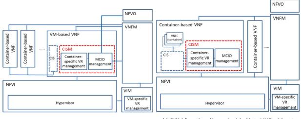
a) CISM functionality embedded into VNF with support for shared container service
