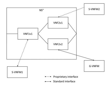
Figure 5.5.2.1-2: In the transitional phase the S-VNFM2 and the G-VNFM operate in parallel managing two different versions of VNF2 belonging to NS"
