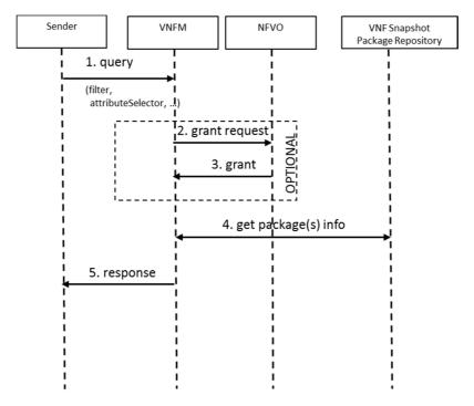
Figure 6.7.5-1: Query VNF Snapshot Package Information Procedure
