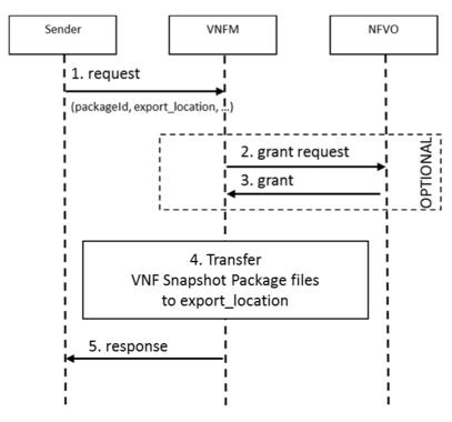
Figure 6.7.3-1: Export VNF Snapshot Package Procedure
