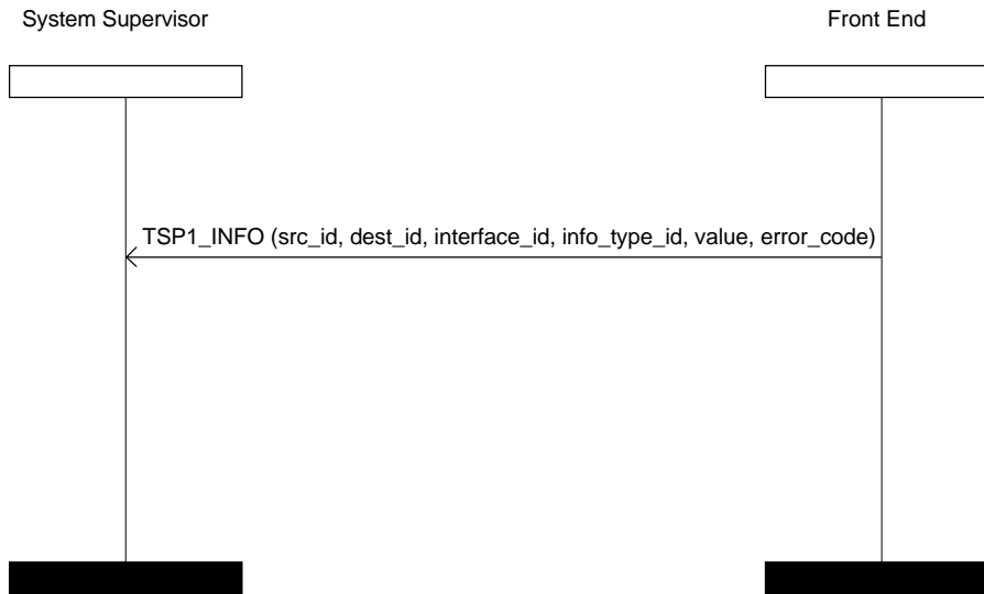
Figure 14: Example of normal operation of the TSP1_INFO PDU to send a message from a Front End to the System Supervisor
