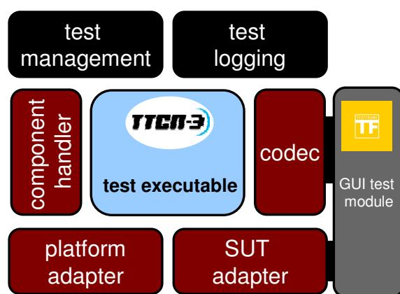
To communicate with GUI applications we have integrated a GUI test module from TestFrame into the TTCN-3 test execution architecture...
