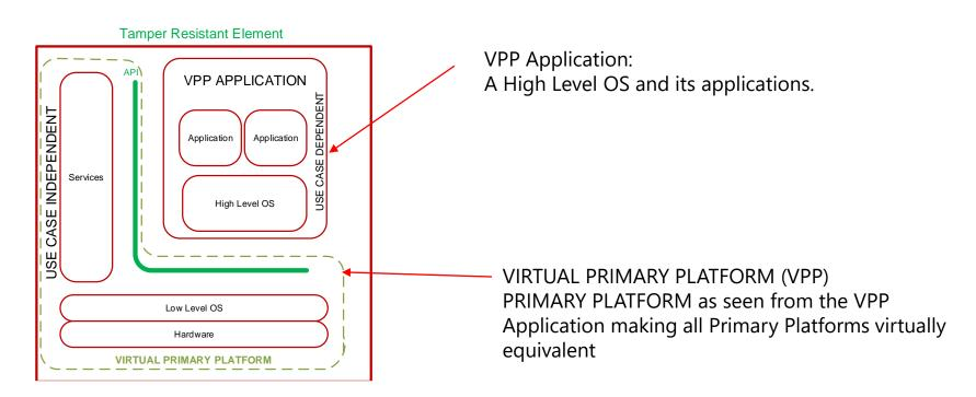
PRIMARY PLATFORM provided by TRE Maker, contains Hardware, Services and Low Level OS with **multi-processing** support
