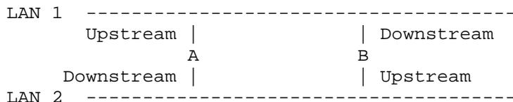
B will unconditionally forward packets from LAN 1 to LAN 2, and A will unconditionally forward packets from LAN 2 to LAN 1. This will cause an upstream loop. A multicast routing protocol which employs a tree building algorithm is required to resolve loops like this.
