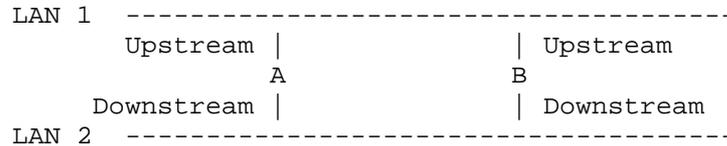
LAN 2 can have two proxy devices A and B. In such configuration, one proxy device must be elected to forward the packets. This document requires that the forwarder must be the IGMP/MLD querier. So proxy device A will forward packets to LAN 2 only if A is the querier.
