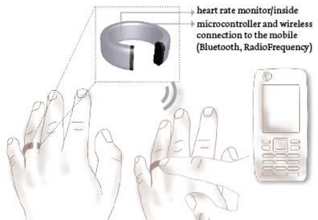
Figure 1: sketch of the ring: To feel the pulse of the partner, the gap in the ring must be filled with the finger.
