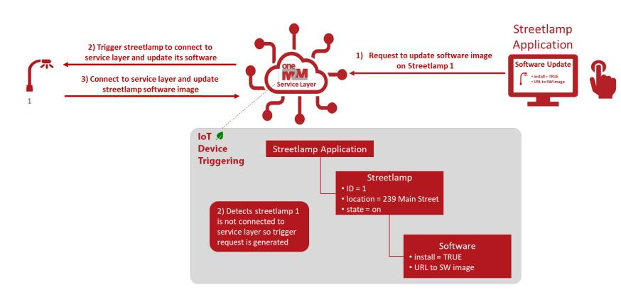
oneM2M device triggering enables an IoT device to "sleep" for long periods of time when not in use, and intelligently "wake up" when applications need to interact with the device.
