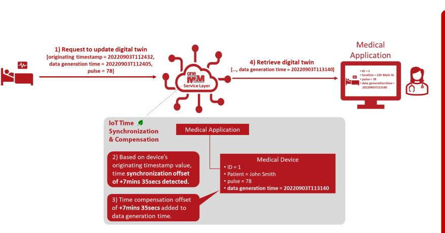
Many resource constrained devices lack the capability to keep their local time synchronized with other devices in the network using traditional technologies such as GPS and Network Time Protocol (NTP).
