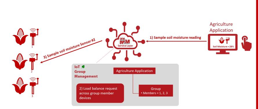
Deploying IoT devices in groups can extend overall lifetime of an IoT deployment and reduce its carbon footprint.
