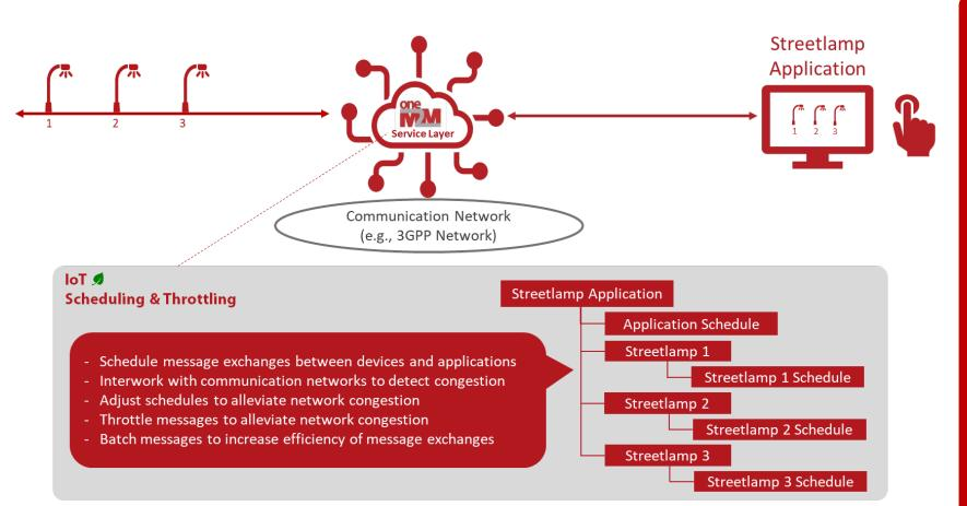
By managing peak demands on communication networks, network operators can optimize the amount of network equipment (e.g., switches, routers, servers, cell towers and base stations) required to meet their customer demands. This can significantly reduce the energy consumption and carbon footprints of their networks.
