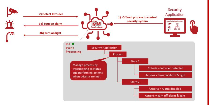
oneM2M supports offloading event detection and processing from devices and applications to the oneM2M service layer.
