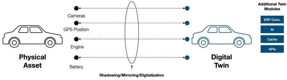
"A Digital Twin (DT) is a comprehensive software representation of an individual physical object. It includes the properties, conditions, and behavior(s) of the real-life object through models and data. A Digital Twin is a set of realistic models that can simulate an object's behavior in the deployed environment. The Digital Twin represents and reflects its physical twin and remains its virtual counterpart across the object's entire lifecycle"
