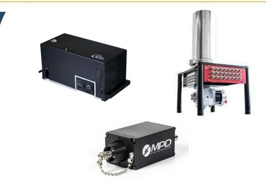
A device that probabilistically transforms the impinging single-photon into a macroscopically detectable electrical signal.
