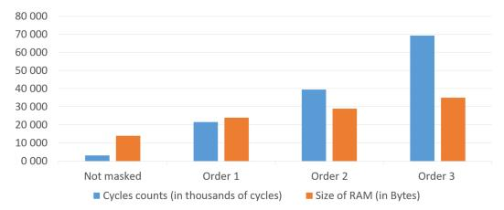
**)** For security order t > 3, required RAM too large for ARM Cortex-M3 target device.
