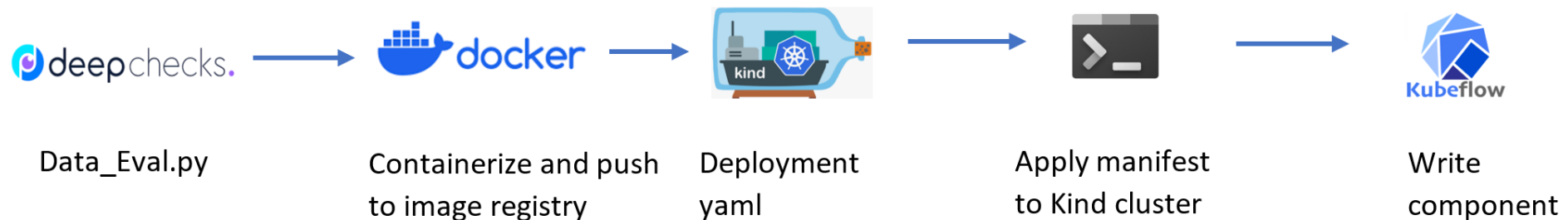
Fig 4.b. Steps to add a data quality evaluation test suite to a Kubeflow pipeline.
