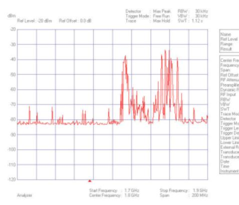
Result - Statuo -Center Frequency Frequency Offset 1.8 GHz D Hz 200 MHz Span Rel Offset 0.0 dB **RF** Attenuator : Off : Low Noise : 50 Dhr Preamplifier Dynamic Range 50 Dhm 30 kHz 30 kHz 1.12 s Max Hold RF Input RBW VBW SWT Trace Mode Max Peak Free Run Detector Trigger Mode Trigger Level Trigger Delay Upper Linit Lower Linit External Reference Disabled Transducer Transducer (dB) 01/01/1995 D.ate Tine :17:24:20 Instrument
