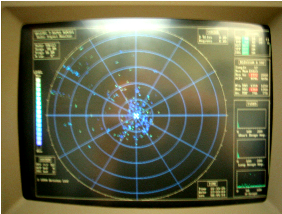
Figure 4: Radar PPI post interference mitigation
