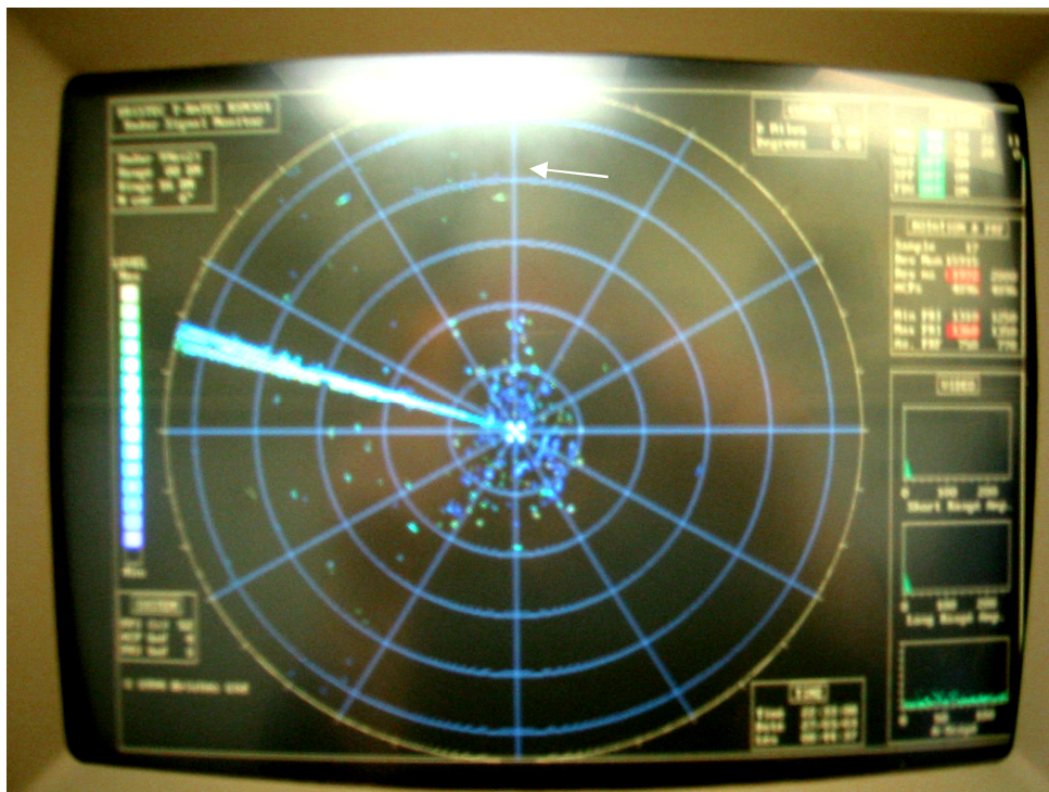
Figure 3: Radar PPI showing interference from wireless LAN
