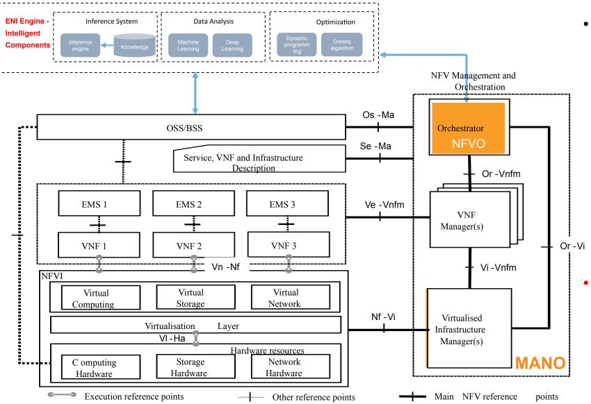
The Network Big Data Analysis module of ENI Engine collects the information of MANO's resource description and dynamic resource to include complete meta-data and data for lifecycle management of the virtual environment.
