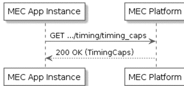
Figure 7.2.5.3.1-1: GET timing capabilities flow
