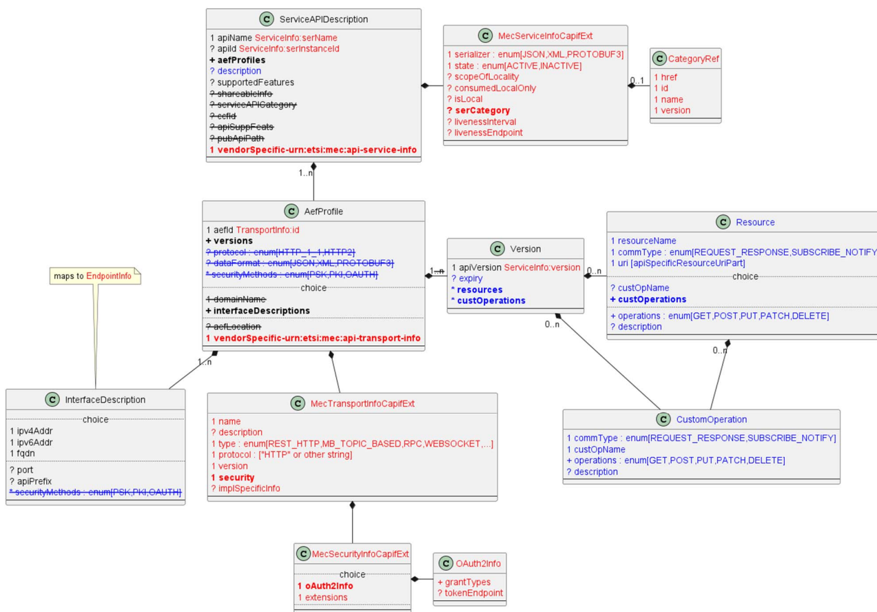
Figure 9.3.2-1: Mapping of the MEC service data model to the CAPIF service data model
