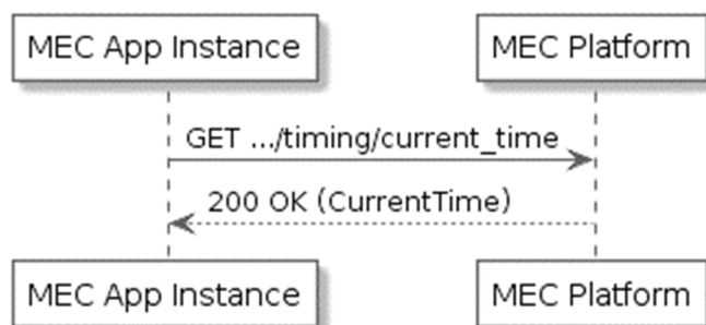
Figure 7.2.6.3.1-1: GET platform time API flow
