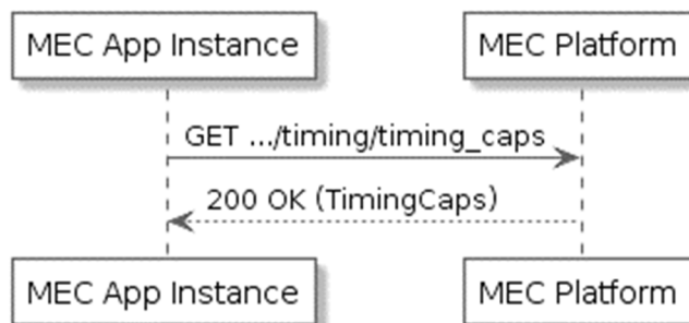
Figure 7.2.5.3.1-1: GET timing capabilities flow
