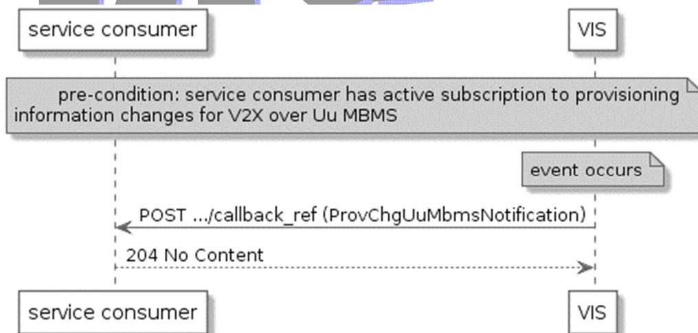
Figure 5.5.8-1: Flow of receiving V2X information event notifications about the provisioning information changes for V2X communication over Uu MBMS
