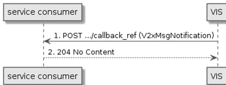
Figure 5.5.10.3-1: Flow of V2X message notification
