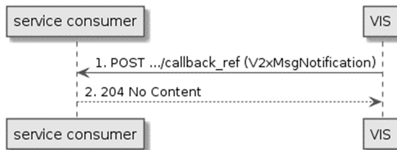
Figure 5.5.10.3-1: Flow of V2X message notification
