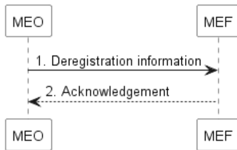
Figure 5.2.2.1.3-1: Information flow of Deregistration
