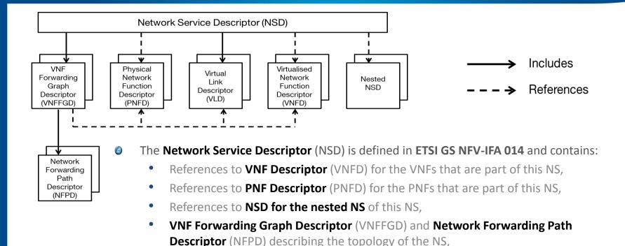
**Virtual Link Descriptor** (VLD) used by NFVO to deploy Virtual Links.
