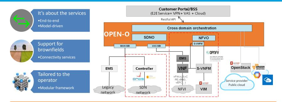
OPEN-O requires unified information & data models that encompass physical, virtual and cloud based infrastructure, SDN & NFV, applications and complex datacenter and intra-datacenter connectivity
