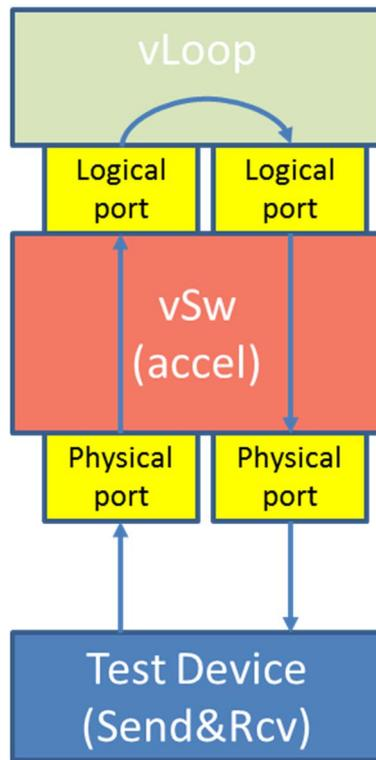
Figure 7.3-2: P - vSw(accel) - (vLoop VNF) - vSw(accel) - P
