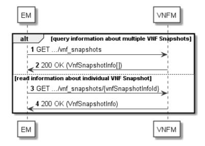
Figure 5.3.15-1: Flow of VNF snapshot query/read
