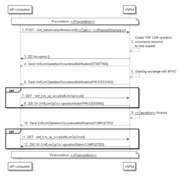
Figure 5.3.3-1: General flow of VNF lifecycle management operations triggered by task resources
