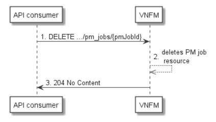
Figure 6.3.3-1: Flow of PM job deletion
