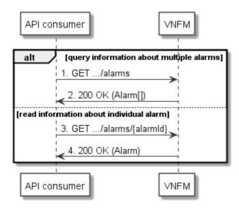
Figure 7.3.1-1: Flow of alarm query/read
