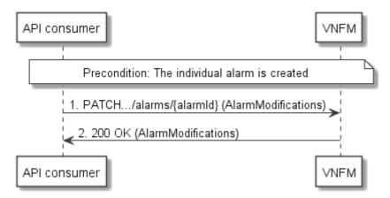
Figure 7.3.3-1: Flow of acknowledging alarm
