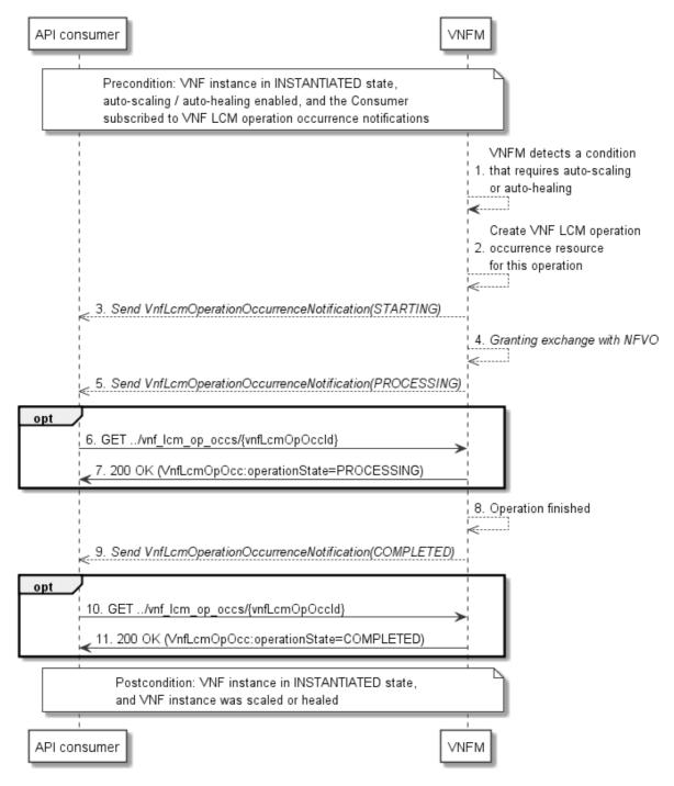
Figure 5.3.4-1: Flow of auto-scaling and auto-healing
