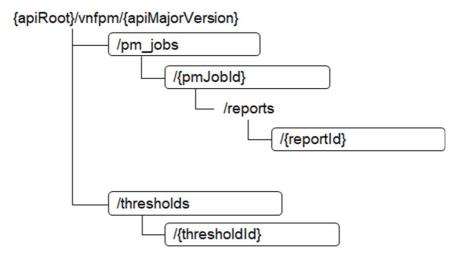
Figure 6.2-1: Resource URI structure of the VNF Performance Management interface
