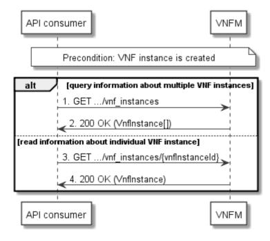
Figure 5.3.5-1: Flow of VNF instance query/read
