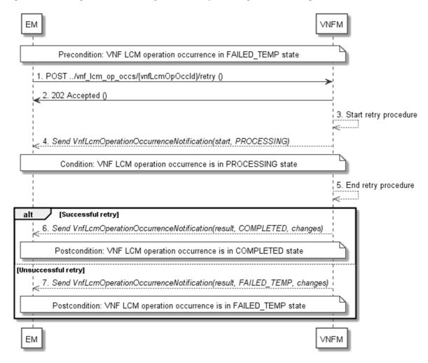
Figure 5.3.10-1: Flow of retrying a VNF lifecycle management operation
