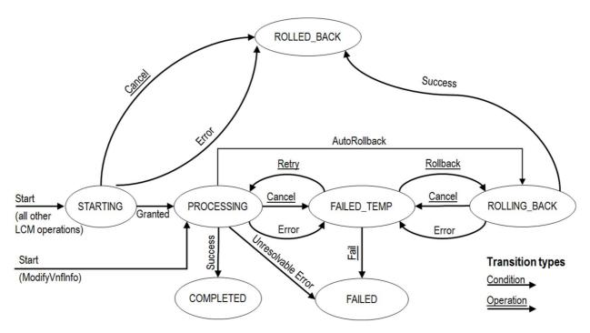
Figure 5.6.2.1-1: States of a VNF lifecycle management operation occurrence
