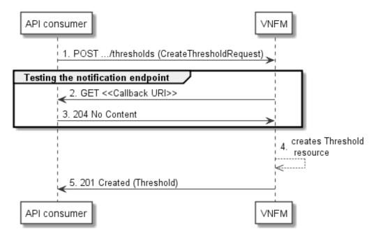
Figure 6.3.5-1: Flow of threshold creation
