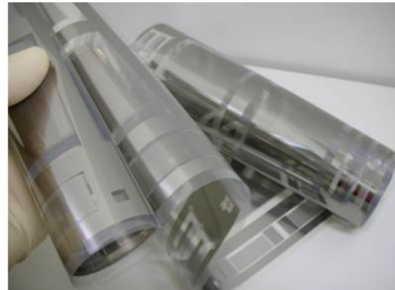
Metal electrode PET base back plane manufactured by roll-to-roll process
