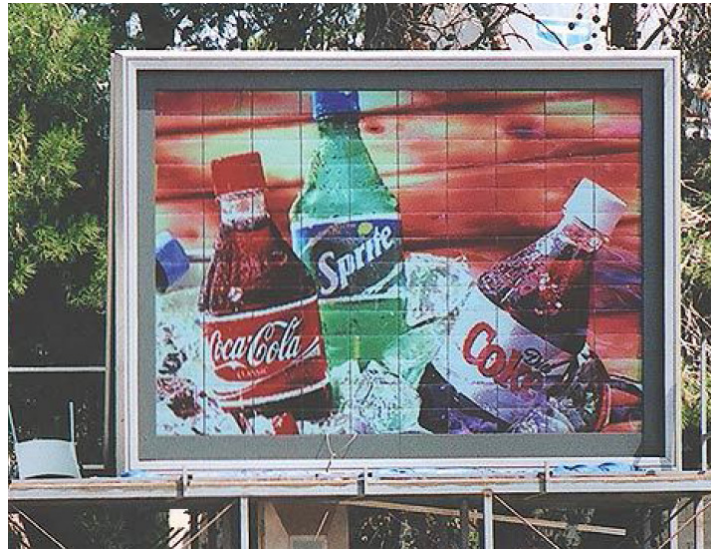
MAGINK tiled ChLCD reflective RGB stacks
